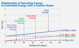
used to build it. In the second chart I show that operating energy (the red dotted line) is greatly reduced when the initial embodied energy (construction – green line) is increased.
